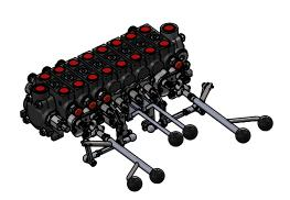
Sectional directional control valve with 8 elements (8ZC70) operated by mechanical joysticks with manual operators controlling 3 spools (3rd movement by rotation). Also available with spool positioners with restrictions (1rAB) for regulating rotor speed.
