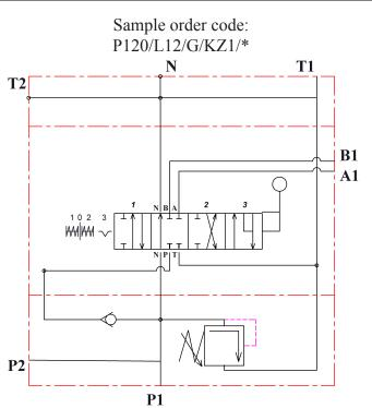
\* The body is specially machined, therefore normal spools A, B, cannot be used!
